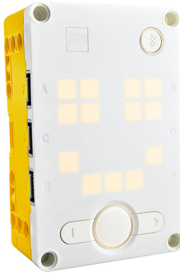
The SPIKE Prime hub – brain, display, buttons, gyro, and lettered ports
