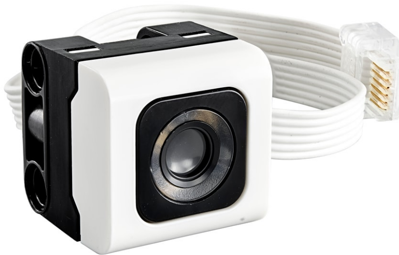
The color sensor – it reads which attachment is mounted
