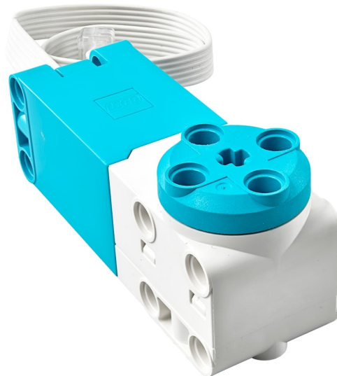
The SPIKE Prime angular motor – the muscle on every port
